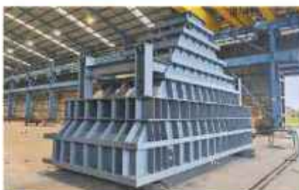
Hopper Chute Smelter Feronike Kolaka Southeast Sulawesi
